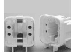
Specifications for Part Number (FL423V-Q3/4):• Quick connect push-in wire terminals for 18 AWG Solid or Twist & Tin stripped 7/16 in.• Rated 75W, 600V. • Each wiring ports excepts 2 wires for easy harness wiring. • Two hole screw mount on base plate.
