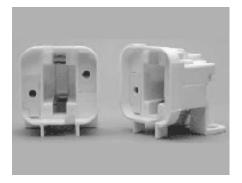
Specifications for Part Number (FL423V-D3):• Quick connect push-in wire terminals for 18 AWG Solid or Twist & Tin stripped 7/16 in.• Rated 75W, 600V. • Two wire ports per terminal to speed harness wiring. • Two hole screw mount on base plate.
