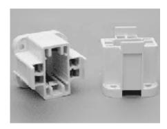
Specifications for Part:• Quick connect push-in wire terminals for 18 AWG Solid or Twist & Tin stripped 7/16 in.• Rated 75W, 600V. • Each wiring ports excepts 2 wires for easy harness wiring. • Four holes on base for secure mounting.
