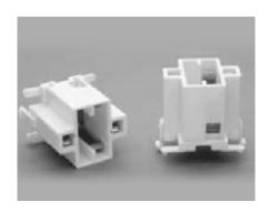
Specifications for Part Number (CF79-VSM):• Quick connect push-in wire terminals for 18 AWG Solid or Twist & Tin or solder dipped wire, stripped 7/16". • Rated 75W, 600V. • Bottom snap-in mount into panel of 0.030-0.067" (0.8-1.7 mm) thickness. • Two wire terminals per wire port.
