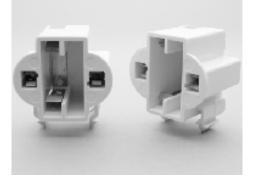
Specifications for Part Number (CF79-HSI): Quick connect push-in wire terminals for 18 AWG Solid or Twist & Tin, stripped 7<sup>1</sup>/<sub>4</sub> Snap-in mount into 0.025-0.040 in. (0.6 - 1 mm) panel thickness in each wiring port accepts 2 wires for easy harness wiring, no extra jumpers or wire nuts to assemble • Rated 75W, 600V.
