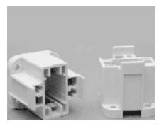
Specifications for Part Number (CF26G24-D3):• Quick connect push-in wire terminals for 18 AWG Solid or Twist & Tin stripped 7/16 in.• Rated 75W, 600V. • Each wiring ports excepts 2 wires for easy harness wiring. • Four holes on base for secure mounting.
