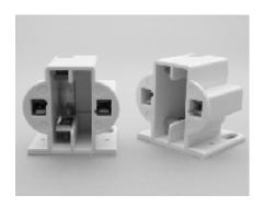
Specifications for Part Number (CF13-HSM): Quick connect push-in wire terminals for 18 AWG Solid or Twist & Tin, stripped 71/416 in. • Snap-in mount into 0.025-0.040 in. (0.6 - 1 mm) panel thickness • Each wiring port accepts 2 wires for easy harness wiring, no extra jumpers or wire nuts to assemble
