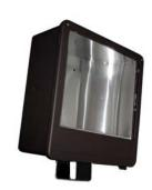
DIE CAST HOUSING & HINGED TOP FRAME WITH SAFETY CABLE RESTRAINT, CHROMATE CONVERSION COATING, TEXTURED BRONZE FINISH, TEMPERED GLASS LENS, PORCELAIN MOGUL BASE SOCKET & BRACKET, CONDUIT ACCESSIBLE ON FIVE SIDES, PHOTOCELL ADAPTABLE
