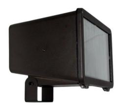
DIE CAST HOUSING & DOOR FRAME, CHROMATE CONVERSION COATING, TEXTURED BRONZE FINISH, TEMPERED GLASS LENS, ALUMINUM REFLECTOR, MOGUL SOCKET (USES STANDARD LAMP VS. REDUCED ENVELOPE), EXTERNAL ACCESSIBILITY WIRING COMPARTMENT, BALLAST MOUNTING BRACKET
