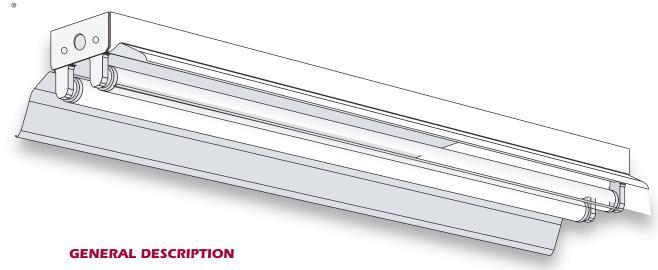
A high quality all-purpose economy Industrial with symmetrical reflector. All fixture parts snap together for ease of installation and maintenance. Side knockouts are included for a convenience outlet, a pull switch and conduit. Sides and back have knockouts for chain hangers.
